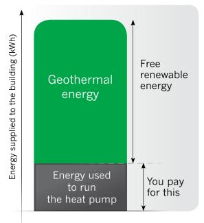
This graphic shows the building's total energy consumption for heating and hot water. The grey area shows the energy used to run the heat pump. The calculation was made for a building of 1 000 m² in an average weather year.
